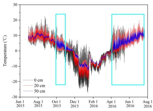
Figure 7. Time series of S1 stream temperatures at depths of 0 cm, 20 cm and 50 cm from July 2015 to July 2016. The green boxes mean the abnormal data in the measure period.
