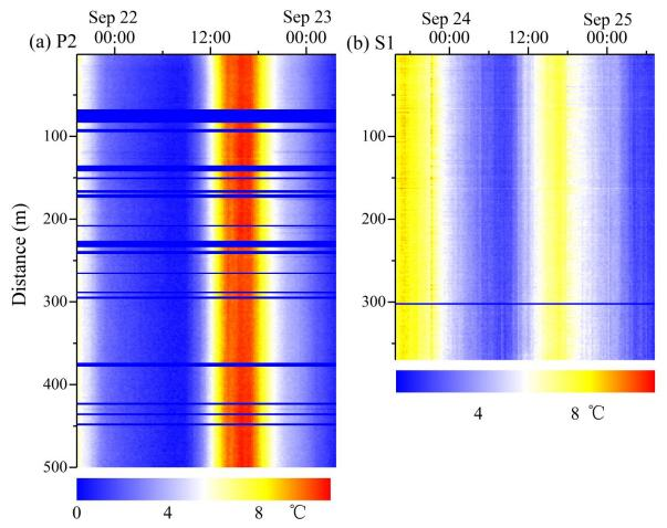
Figure 5. Riverbed temperatures measured by FO-DTS at (a) P2 (from 19:00 Sep 21 to 03:00 Sep 23, 2015) and (b) S1 (from 15:00 Sep 23 to 07:00 Sep 25, 2015).
