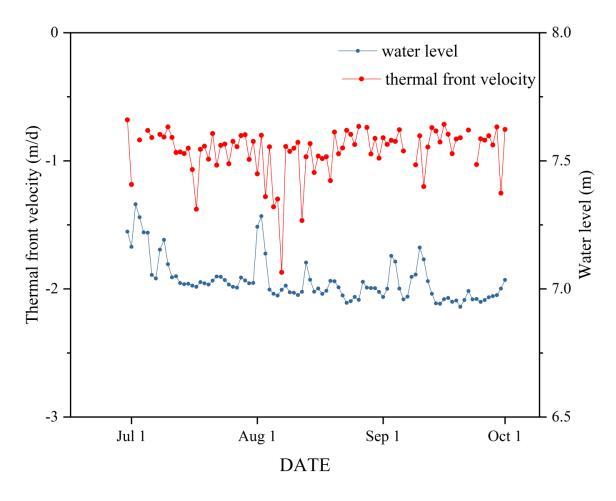
Figure 9. Time series of thermal front velocity and water level changes at S1 from July to September in 2015.
